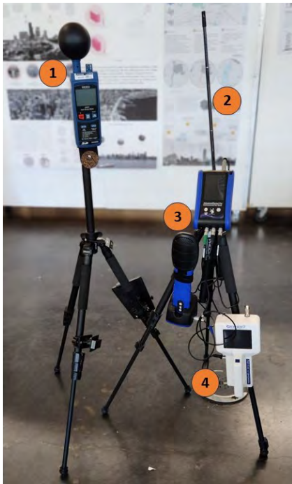
Figure 2: Equipment setup used by the students to collect data required for accessing thermal comfort and IAQ in the design studio. List of the devices: 1-Heat Index Meter, 2-Air Velocity Meter, 3-Gases Meter, 4- Particulate Matter Meter.
