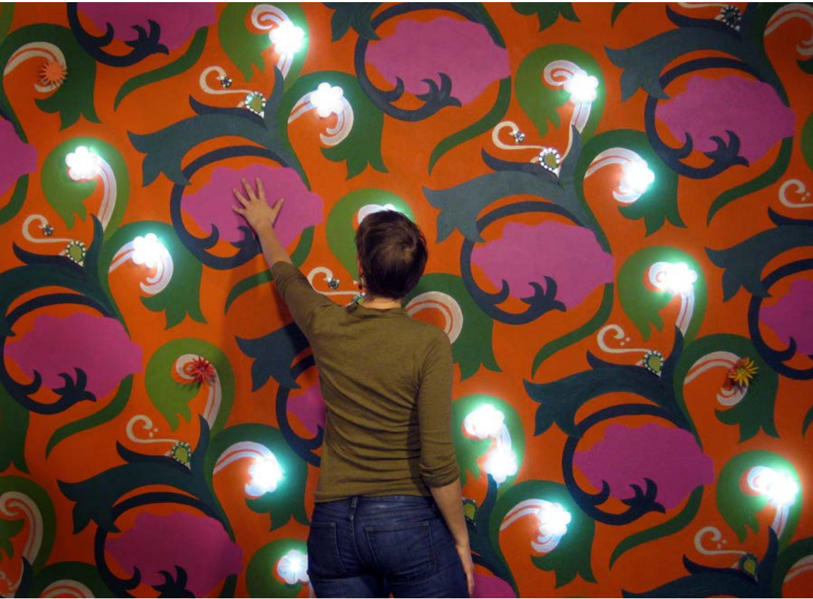
Fig. 7. Living Wall. An interactive wall painting made from conductive paint, magnetic paint, traditional paint, and custom circuit boards. Developers: Leah Buechley, David Mellis, Bonifaz Kaufmann, Hannah Perner-Wilson, Emily Lovell, and Kanjun Qiu, Tshen Chew, and Jie Qi of the MIT Media Lab. 2009. Photo © Leah Buechley. http://highlowtech.org/?p=27 .
