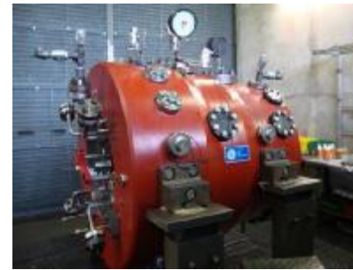
Figure 4a. Leakage test arrangement of high pressure barrel compressor
