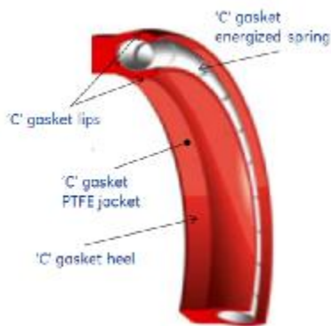
Figure 2. 'C' gasket schematic
