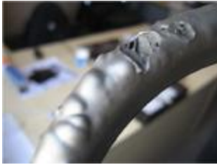
Figure 1. Damaged O-ring caused by explosive decompression
