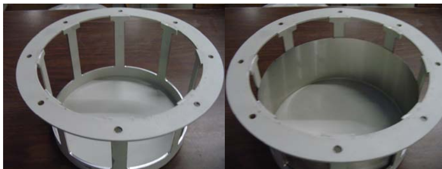
Figure 24. Internal Fractionators – L) 581 cm 2 , R) 290 cm 2 .
