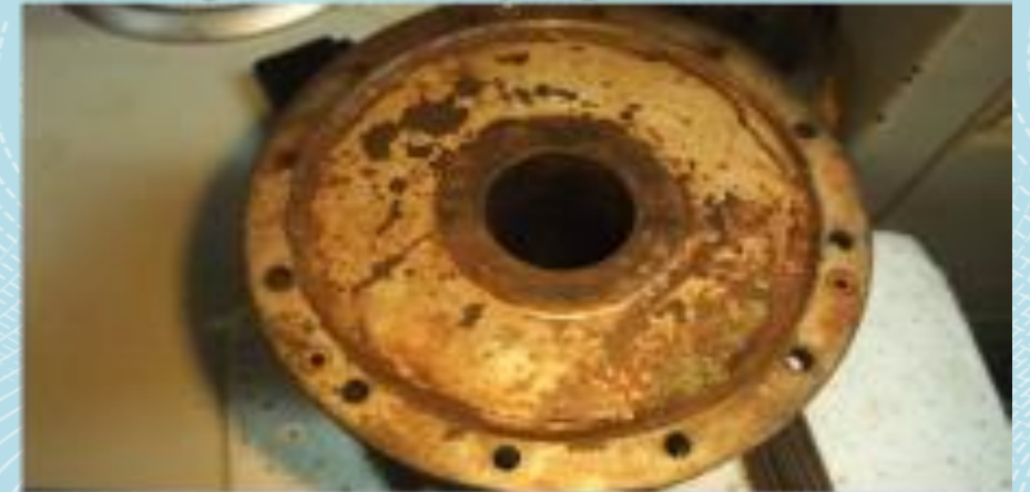
Location of August 15 MB Coupling Failure
