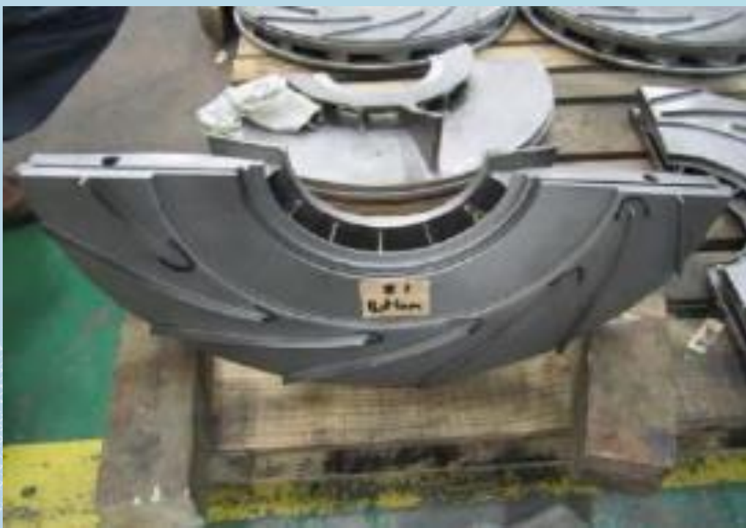
HP Inlet Diaphragm (bottom)
