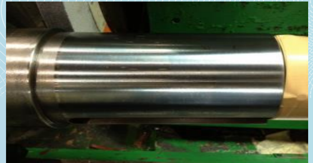
Completed Surface Finish (roughness 0.266 micron)
