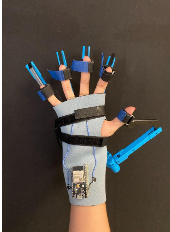
Figure 11. Custom-made Vibration Glove and SenseGlove
