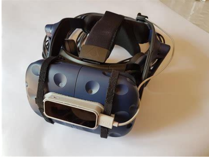
Figure 2.3: Example from Leap forums [19] of sensor mounted using 3D printed mount
