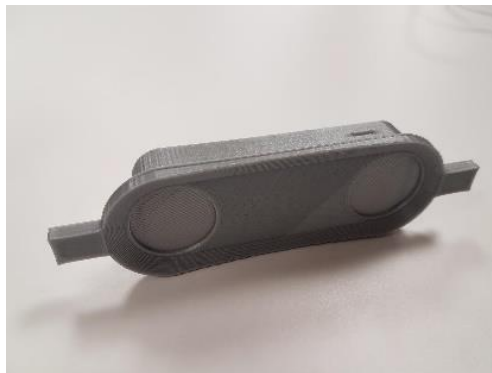
Figure 2.2: 3D printed mount for HTC Vive Pro headset
