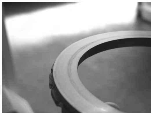
Figure 8. Scratched static seat.
