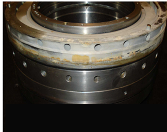
Figure 7. Salty deposit on gas seal housing.
