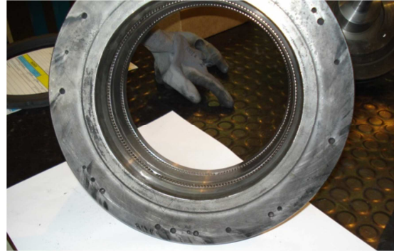
Figure 6. Black powder coming from compressor inner labyrinth.
