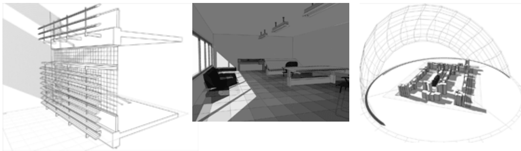
FIGURE 5 Output from Autodesk Ecotect Analysis 2010 showing, sunlight entering window, day lighting model and shadows and reflections
