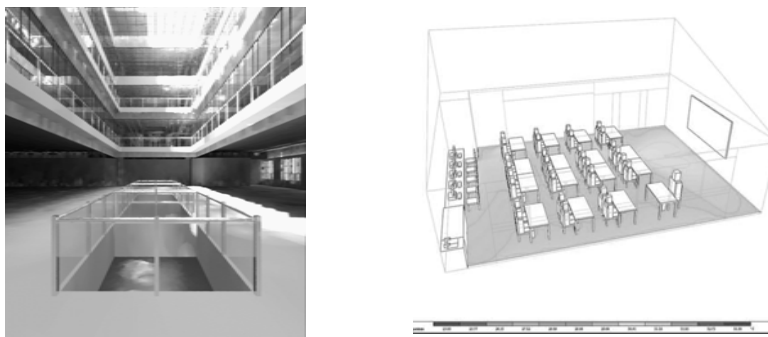
FIGURE 10 Output from IES <VE> showing day-lighting and comfort analysis (Integrated Environment Solutions)
