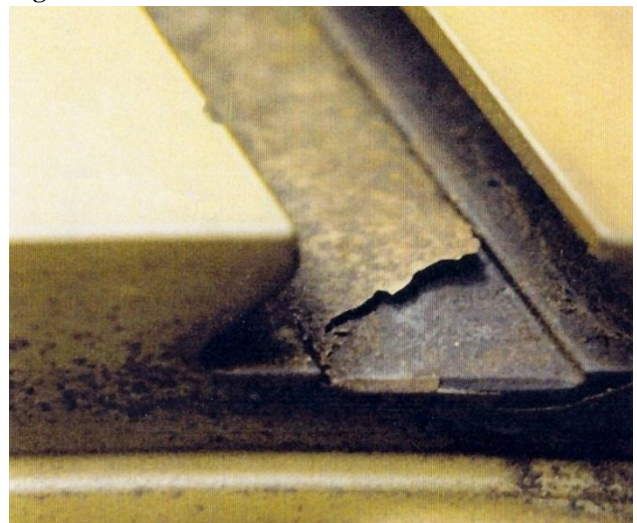
Figure#16 - Disk Coating Delamination -18 months
