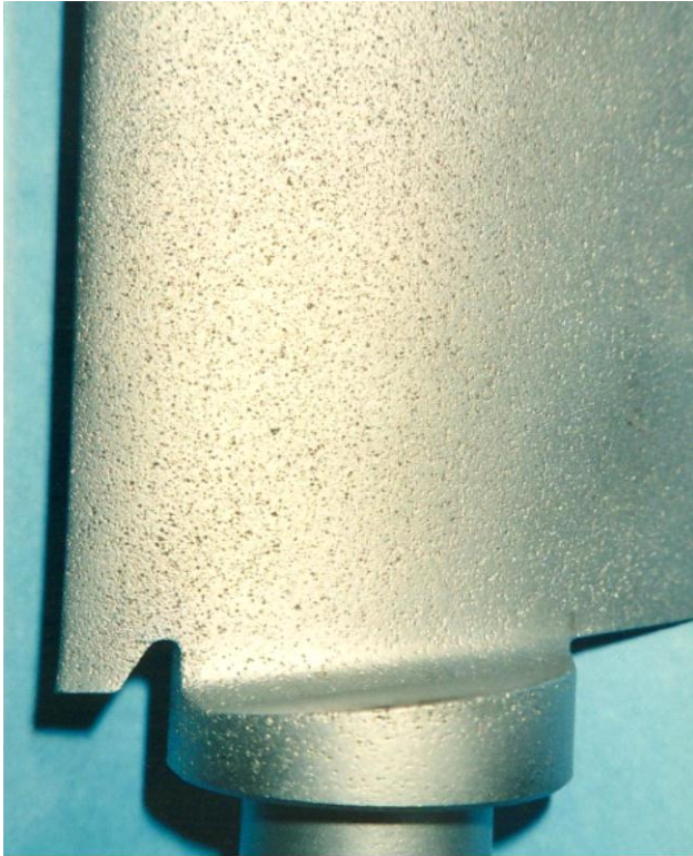
Figure #1 – Corrosion Pitting of 410 SS IGV after 36 months of service
