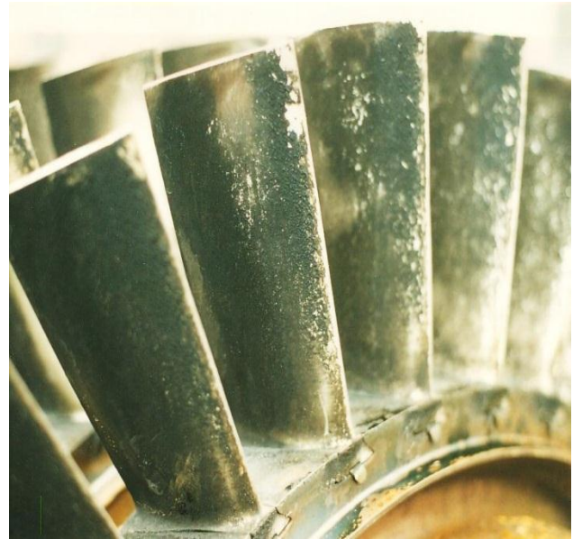
Figure #19 – Typical Inlet Stage Flow Path Deposits
