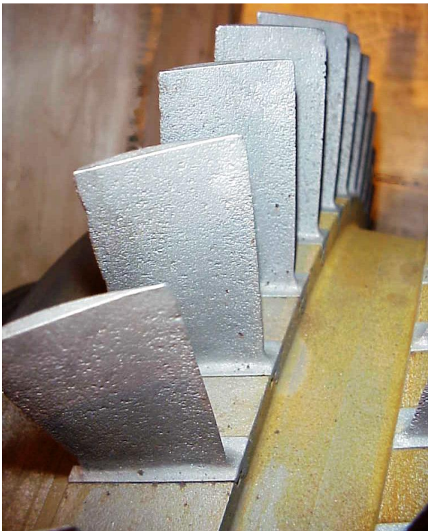
Figure #2 – General and Pitting Corrosion of 403 SS First Stage Rotor Blades after 24 months service
