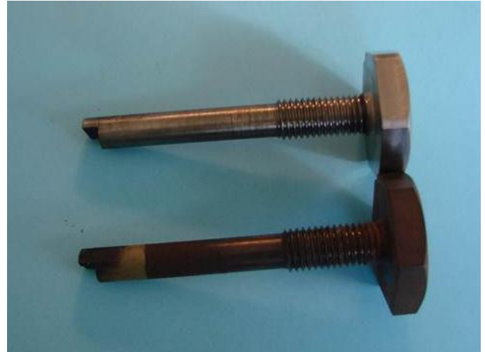
Figure #8 – As received Titanium (top) and Coated Alloy Steel (bottom) Corrosion Coupons
