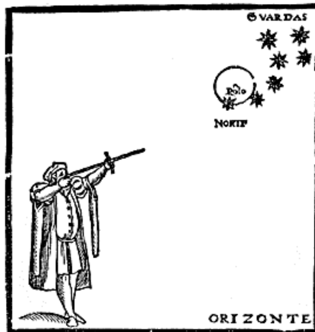
Fig. 4.8. Sighting Polaris with a cross-staff from Medina (1545). (After Medina 1545)
