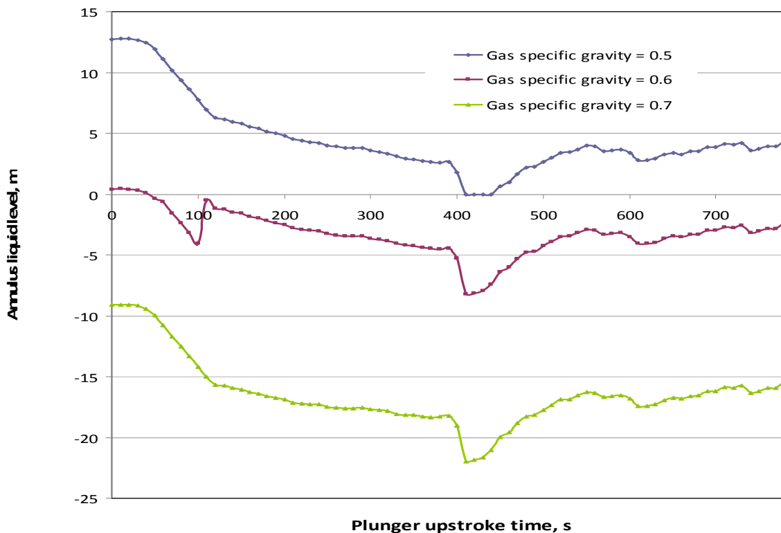
Figure 5.4 – Comparison of Annulus Liquid Levels for Three Different Guesses of Gas Specific Gravities
