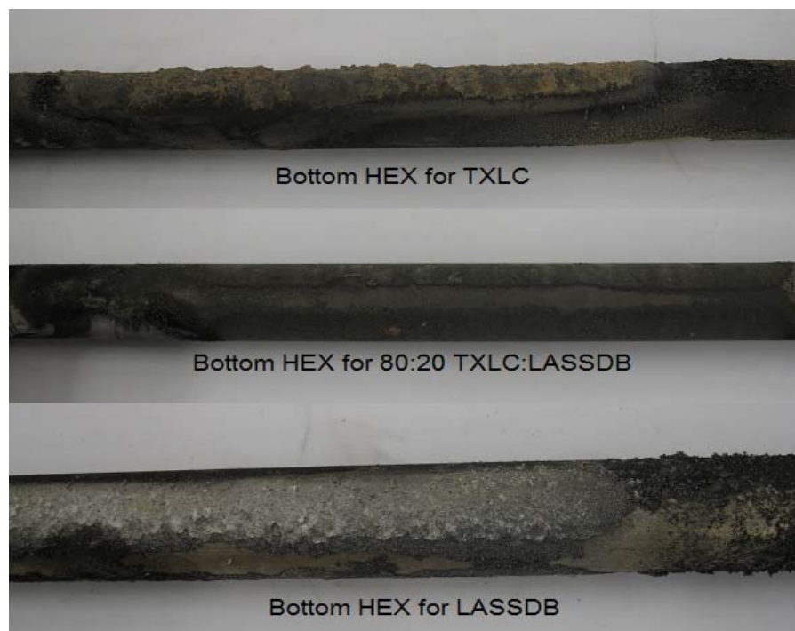
Figure 7.13. Ash depositions on bottom HEXs for several reburn fuels.
