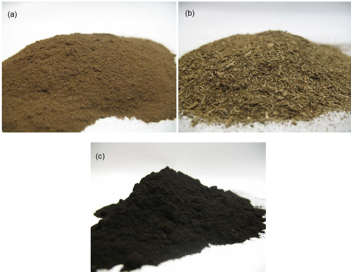
Figure 5.2. Fuel samples used in CB reburning: (a) LAPCFB, (b) LASSDB and (c) TXLC.
