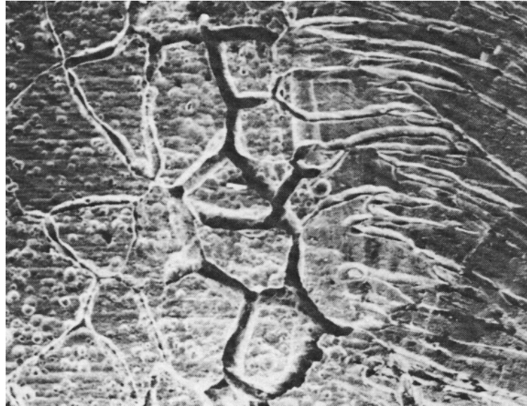
Figure 2.11 Intergranular corrosion in austenitic stainless steel [20].
