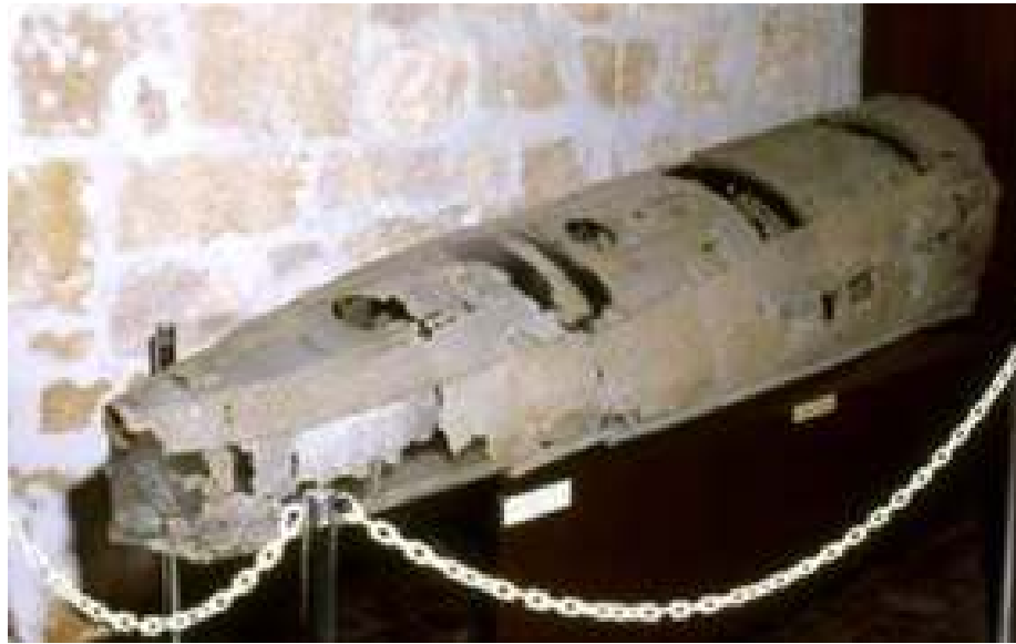
Figure 1.3 The Junker's W33 showing extensive pitting corrosion on the skin.
