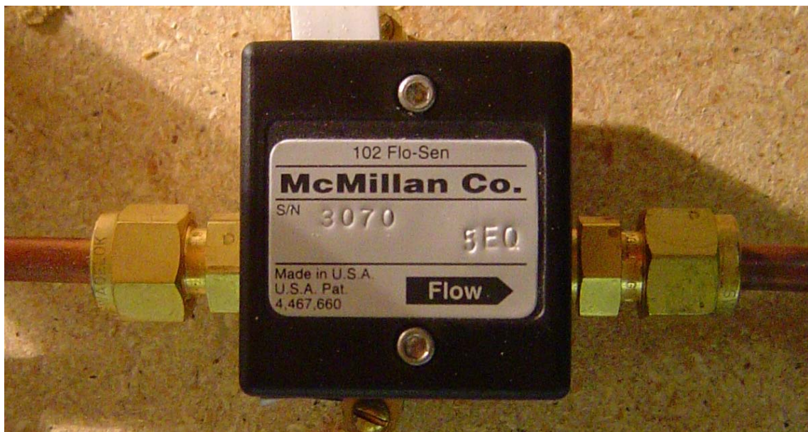
Fig. 2.28 Refrigerant flow transducer
