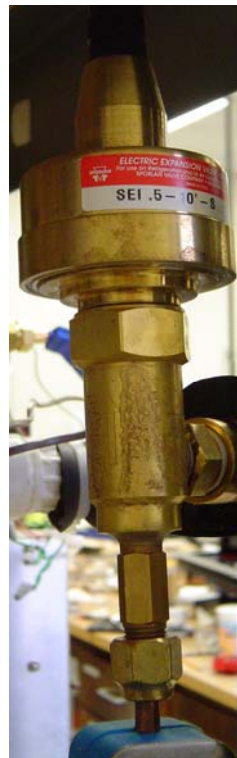
Fig. 2.14 Electronic expansion valve (EEV)
