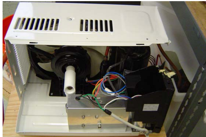
Fig. 2.7 Condenser water chiller
