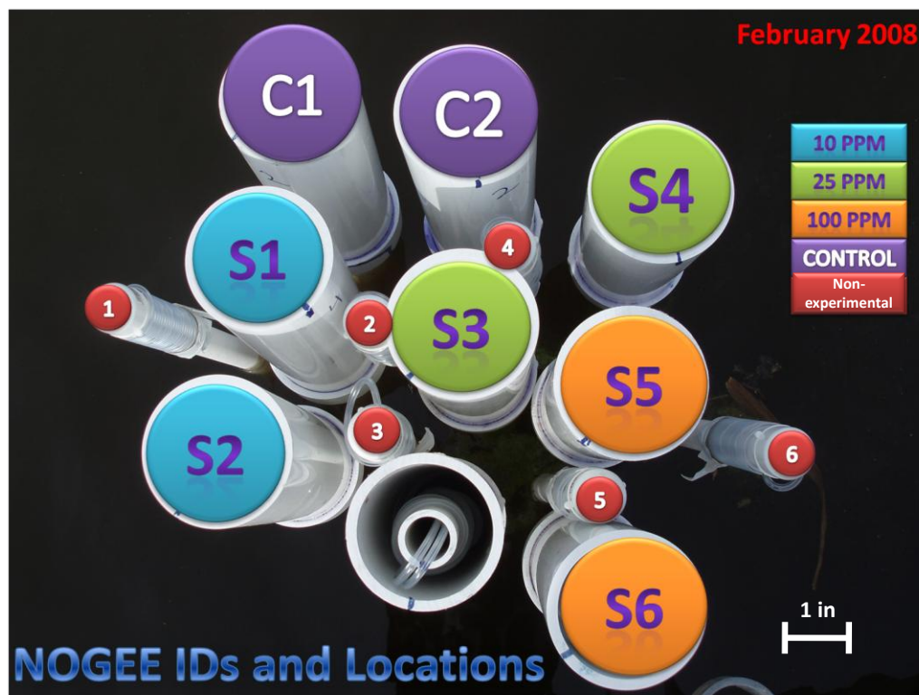
Figure 5.1. NOGEE placement for February 2008 experiments. October 2007 NOGEEs were conducted in the same vicinity and with similar spacing. Non-experimental NOGEEs (small wells) provided initial sponge samples for molecular analyses of the microbial population.
