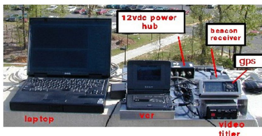
Figure 2.1. The major off-the-shell components of the portable airborne laser system (PALS) (Photos courtesy of Dr. Ross Nelson of NASA).
