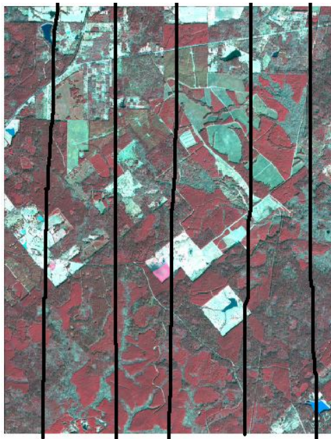
Figure 3.2. Parallel transects flown by a profiling LiDAR (profiler) over a study site: the dark lines are the flight lines of the laser profiler, the background is a false-color QuickBird image.
