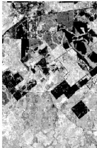
Figure 5.10. LiDAR-derived LAI map with a spatial resolution of 35 m; it was generated by using the LPM predictor r_{in+grd/total} .
