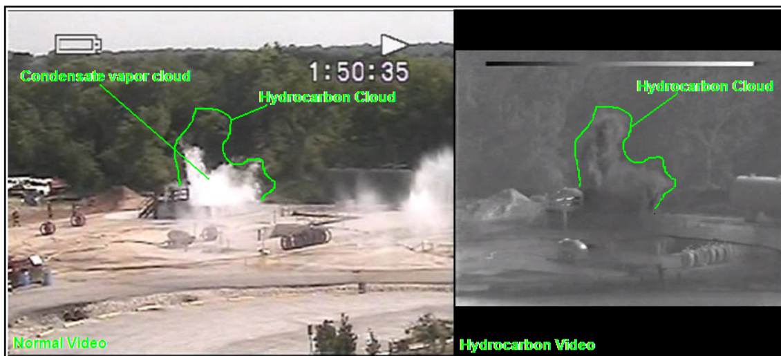
Figure 20. Comparison between condensate and hydrocarbon vapor cloud (Courtesy of Michael Moore, Flameout)
