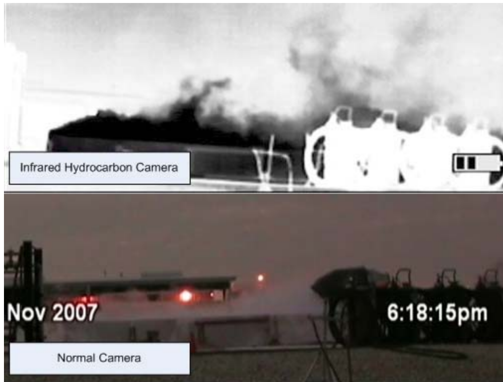
Figure 62. Video picture of release on concrete with normal and infrared hydrocarbon camera
