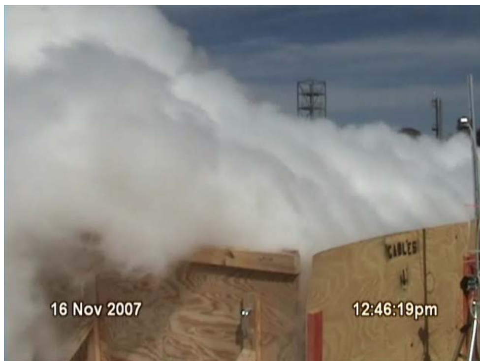
Figure 46. Illustration of interaction between the edge of the wall and the condensate cloud
