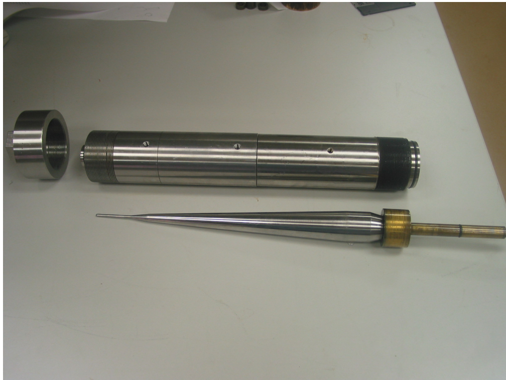
Fig. 3.5—Inner pin and outer casing of the prototype laminar flow viscosity sensor.
