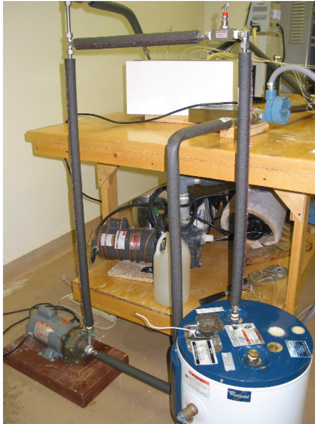
Fig. 4.7—Storage tank and pump connected to the experimental flow loop.
