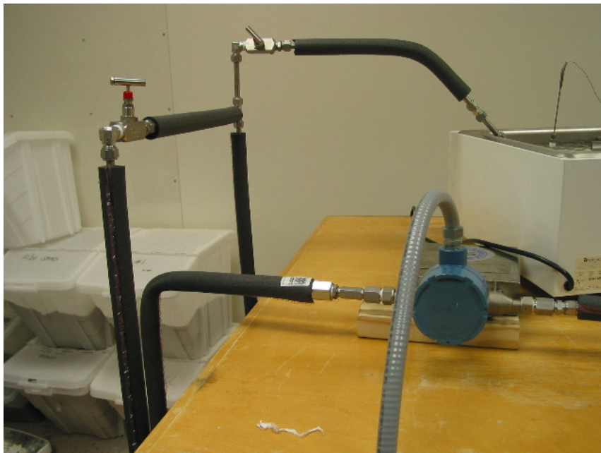
Fig. 4.6—Flowmeter attached to the experimental flow loop.
