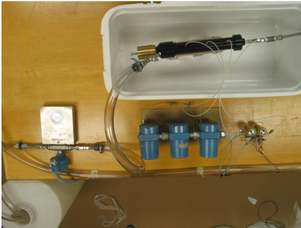
Fig. 4.2—Viscosity sensor, flow meter and pressure transducers installed the preliminary experimental flow loop.
