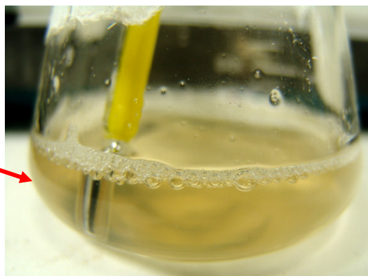
Figure 30: 10 wt% of xanthan and cellulose enzymes prepared in PFB solution
