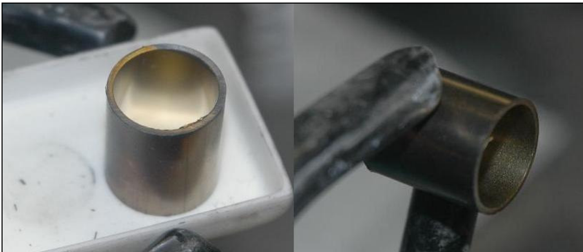
Figure 8. Golden color of experiment 24 indicating nitride contamination.
