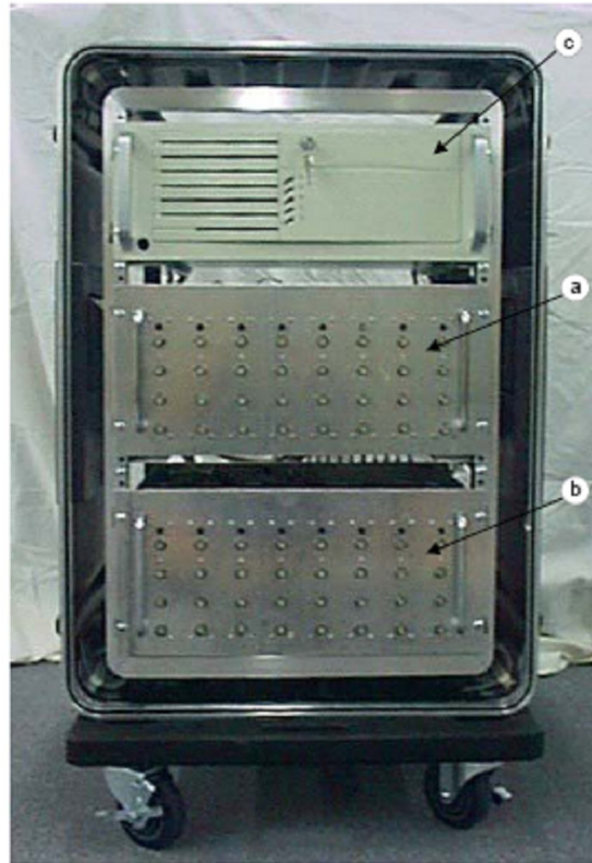
Figure 2.10: The 200MHz signal obtained from the SEA coil is mixed down to an IF of 500KHz. Components (a) and (b) contain 32 IF receiver channels. The data acquisition computer (c) is equipped with 64 channel digitizers.
