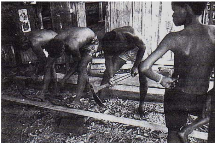
FIGURE 8-7. Brazilian boat builders adzing individual planks (After Carrell and Keith 1992:291)
