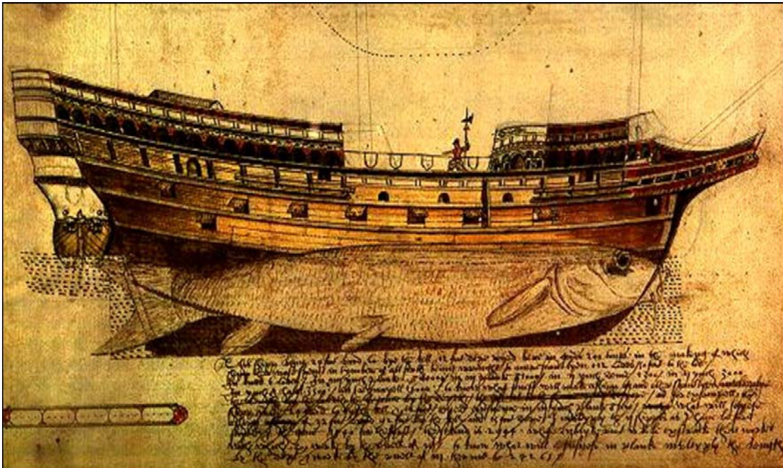
FIGURE 6-1. The body of a fish superimposed over the hull of a ship (After Kemp 1988:31)
