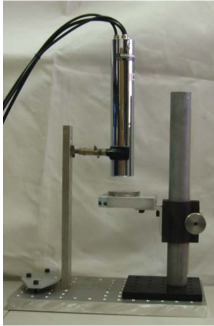
Figure 3: Image of the NaI(Tl) wound counting system.
