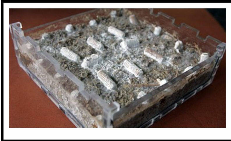
Figure 2. Mushroom/perlite composite insulation growing in a dish (Chua, 2007).
