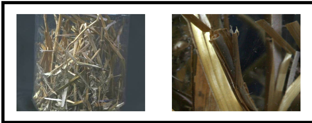
Figure 16. Straw with 0 mL of water after 35 days.
