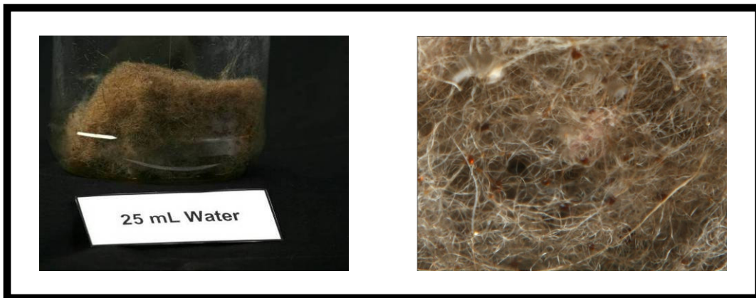
Figure 11. Wool with 25 mL of water after 35 days.
