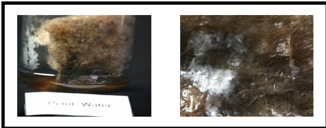
Figure 12. Wool with 75 mL of water after 35 days.
