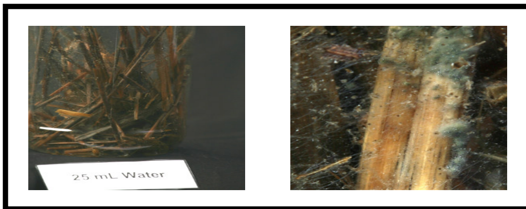
Figure 17. Straw with 25 mL of water after 35 days.
