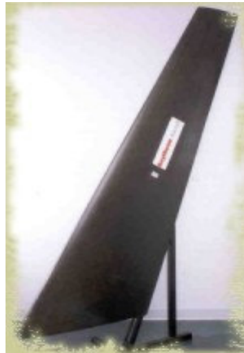
Figure 1.1. Aircraft horizontal stabilizer (www.braider.com).
