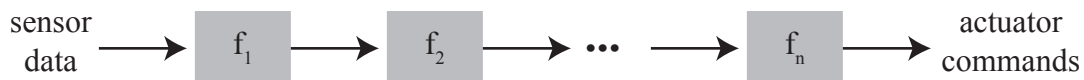
Fig. 6. A control scheme that uses n processing steps to process sensor data and generate an action. Each step requires the others and can not, in isolation, control the agent.
