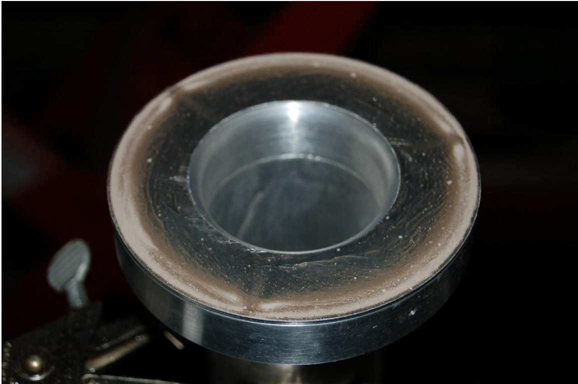
Figure 26: Fine ARD collected on a grease coated impactation plate in an IRI-100. Some dust is wetted by the grease but excess dust is sitting loosely on top of the other particles in the outer region of the collection surface, which is under the impactation jet.
