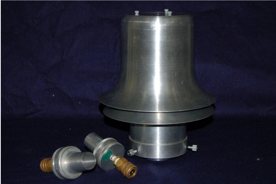
Figure 14: Photograph of BSI-100 IRI and isokinetic nozzles used in experiments.
