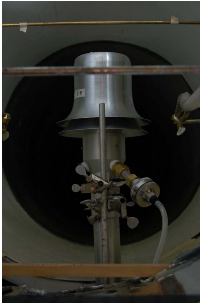
Figure 8: Photograph of placement of BSI-100/IVI-400 in wind tunnel.
