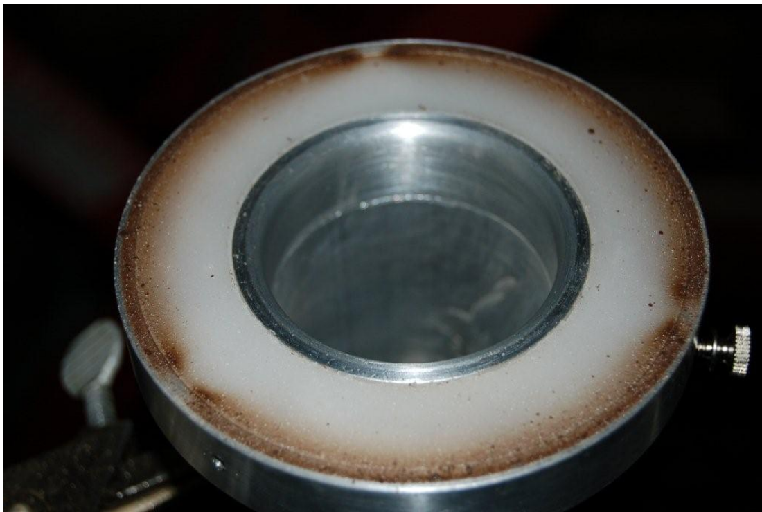
Figure 27: Fine ARD collected on an oil soaked porous media collection surface in an IRI-100. All particles are fully wetted by the oil.
