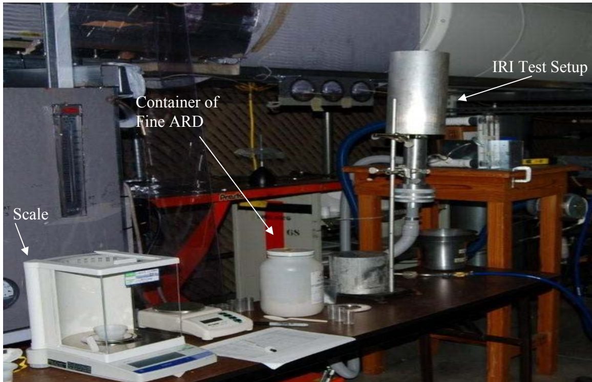
Figure 11: Photograph of test setup of static load testing. Pictured here are the scales used to measure dust mass, a container of Fine ARD, and the IRI setup for this test.
