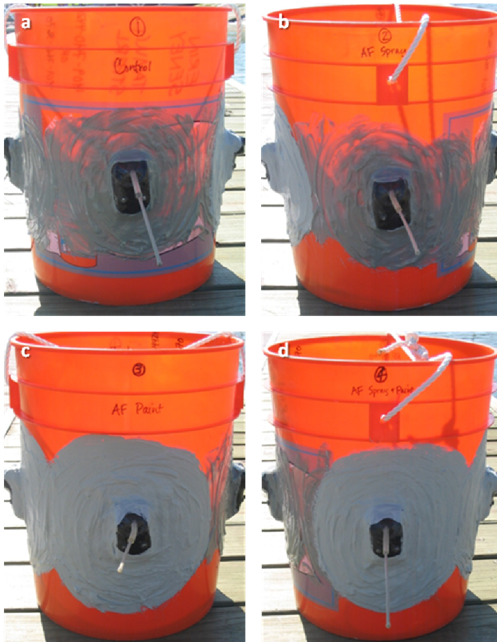
Fig. 6.3. Biofouling trial. Treatments on bucket: (a) control, (b) spray-on anti-fouling paint, (c) brush-on antifouling paint, and (d) both antifouling paints. Photos by E. Seney.
