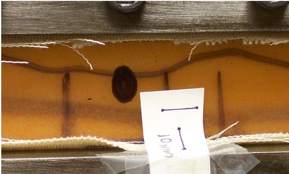
Figure 57. Picture 3 for Specimen #2 shows the dot's ellipsoid shape at about 58% deformation.
