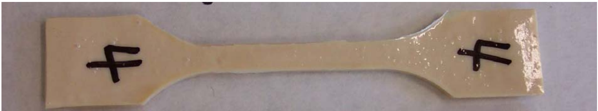
Figure 41. An ASTM D638 specimen from FMSC 1035T ® resin is shown after fully cured. The dates when the specimen made have been recorded for every specimen.
