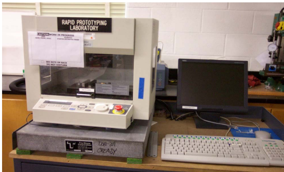
Figure 10. Roland PNC-300 ® mini-CNC machine. This machine cut the wax mold for specimens.
