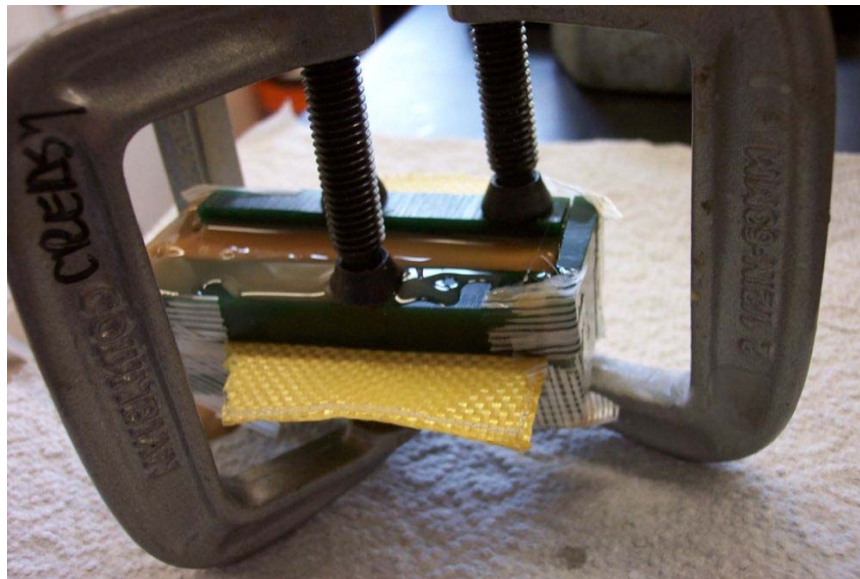
Figure 33. Actuator is in curing process with soft polyurethane resin. A clamping device put forces to make sure the parts in appropriate place during curing.
