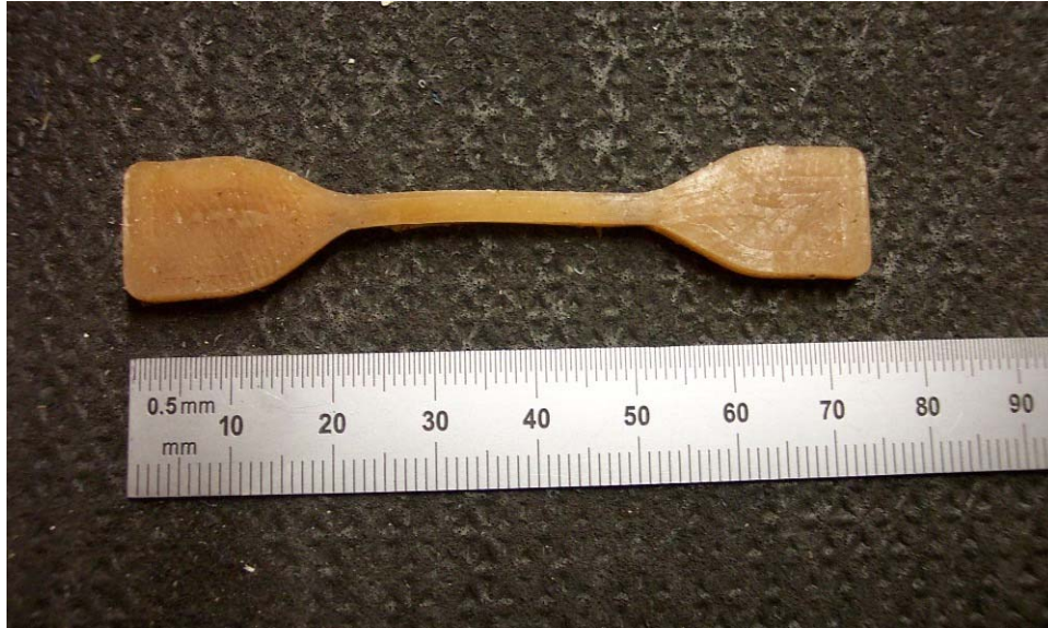
Figure 12. A dog-bone shaped specimen used for tensile test.
