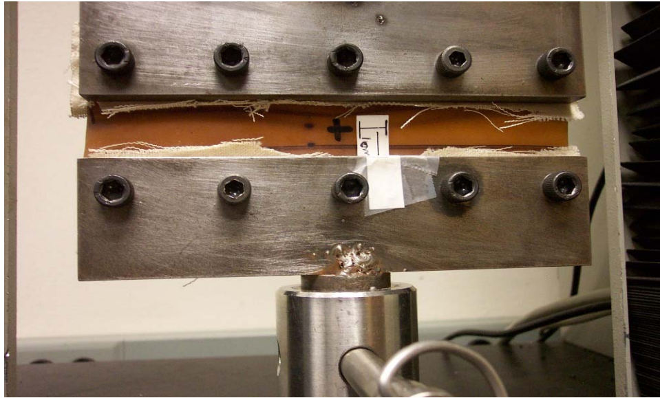
Figure 50. Picture 1 shows the planar tension-pure shear test for Specimen #1. The small cross in the center of the specimen shows the deformation state of planar tension that is equivalent to pure shear. The marker to the right of the small cross is a reference for image analysis.
