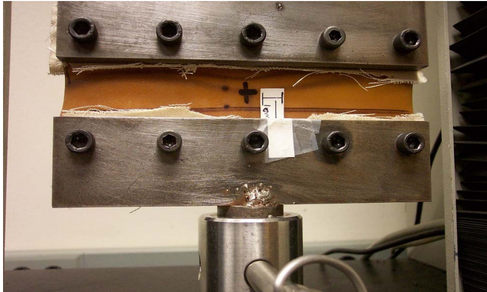
Figure 51. Picture 2 shows Specimen #1 at larger stretch. This shows about 26% deformation.
