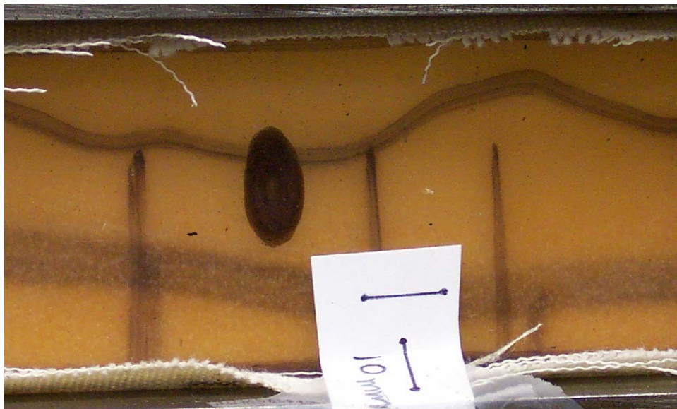
Figure 59. Picture 5 for Specimen #2 shows the dot with the crosshead stopped at about 108% deformation; this is the maximum deflection applied.
