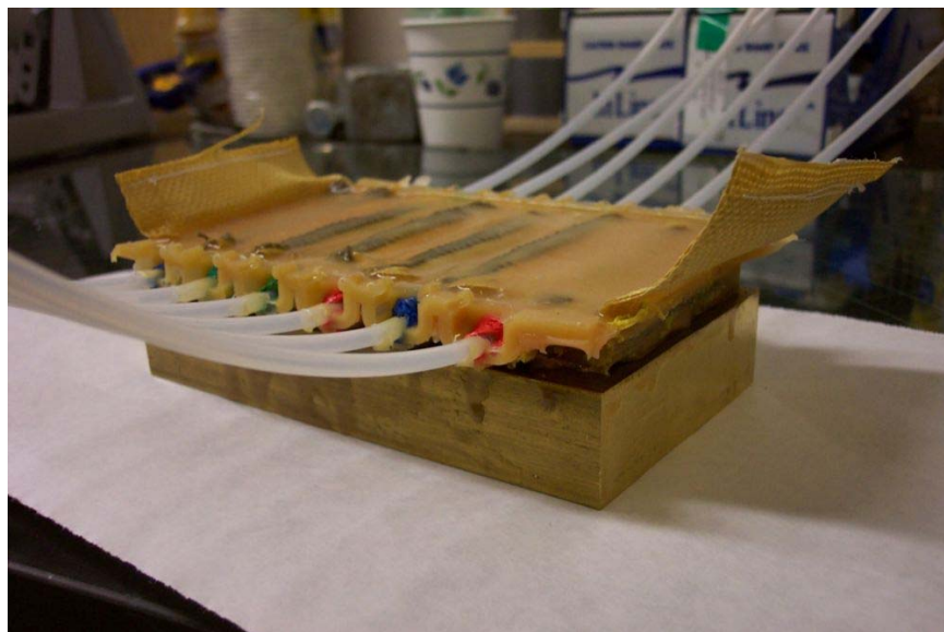
Figure 36. A shear actuator panel with 12 elements is fabricated. It is bonded to aluminum base.
