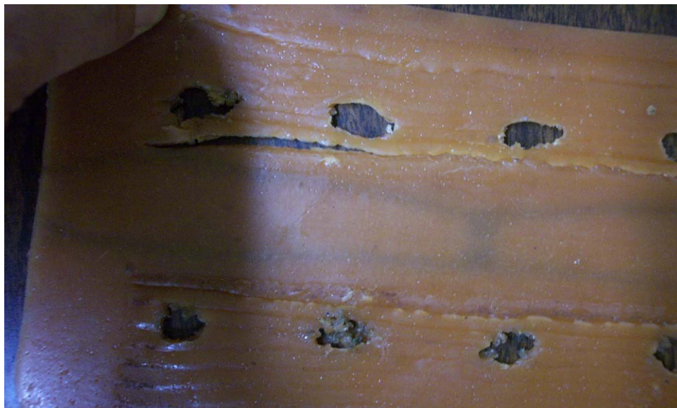
Figure 48. Sharp edges in the wide grips cut the specimen during initial work.
