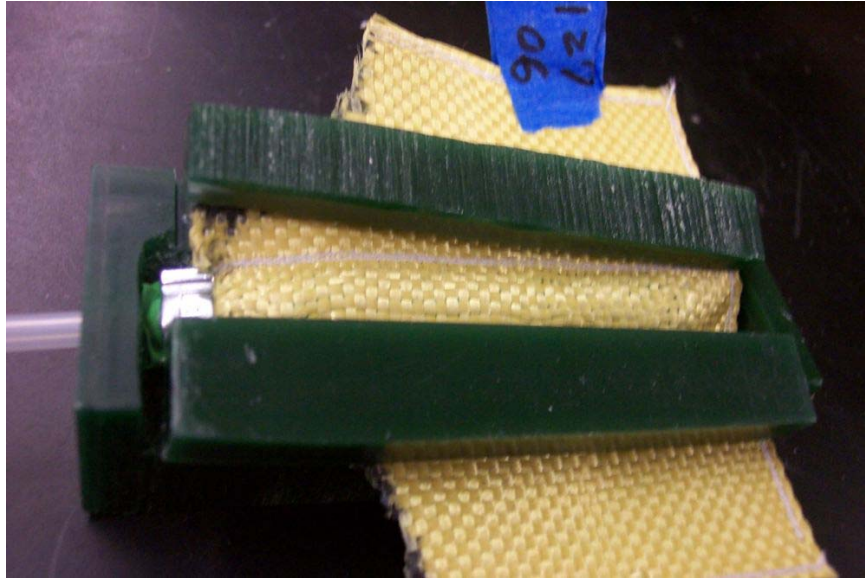
Figure 32. The mold and Kevlar fabric element set up to apply the soft polyurethane resin.
