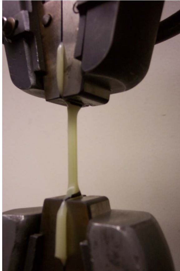
Figure 37. The dog-bone shaped specimen mounted to the crossheads.
