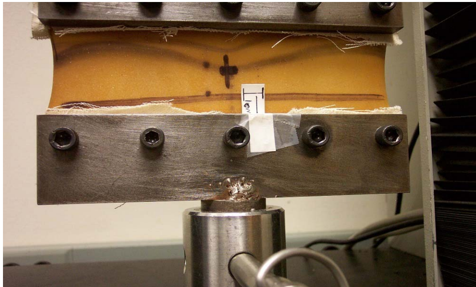
Figure 54. Picture 5 for Specimen #1. The crosshead movement stopped at about 103% deformation, took this picture, and started in reverse direction to record downward curve.
