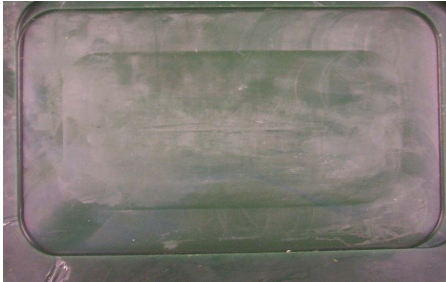
Figure 13. Wax mold made the planar tension specimen.
