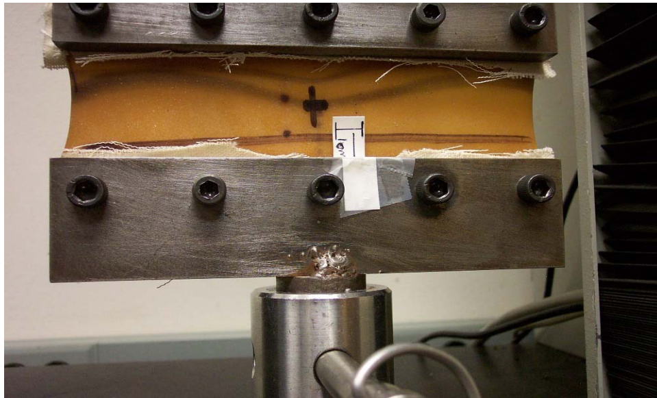
Figure 53. Picture 4 shows Specimen #1 at about 78% deformation.
