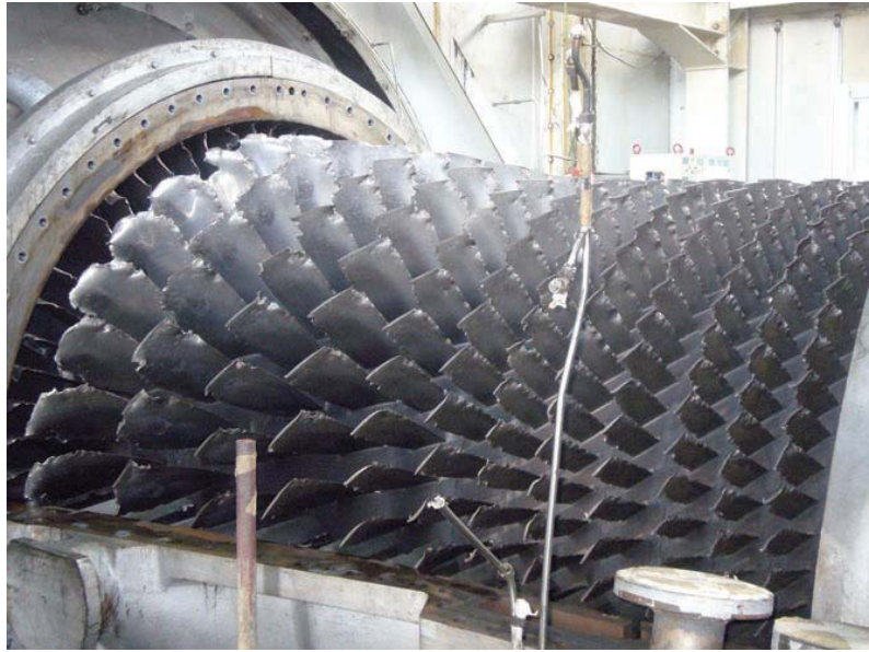
Figure 1.1 Failure of a first-stage blade damages all subsequent stages. 1
