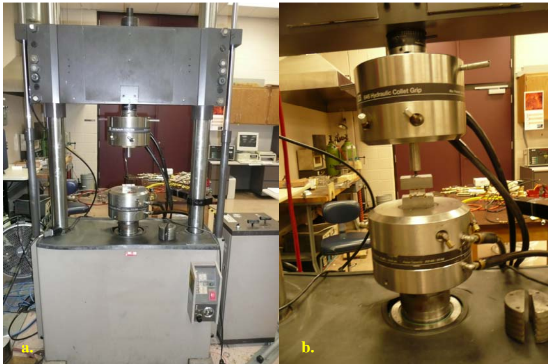
Figure 4.2 (a) MTS 100 kip cyclic loading machine and (b) four-point bending setup.
