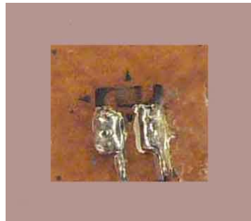
Figure 3 A close-up view of a uniaxial strain gage
