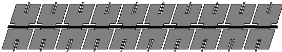
Figure 2.13 Microstrip based UC-PBG structure. Metal 5 was used for the microstrip line and Metal 1 for the UC-PBG ground plane.
