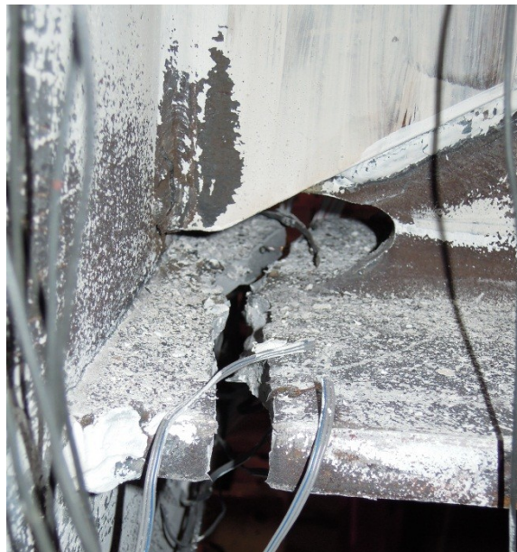
Figure 5.84 Photo of the east beam bottom flange of Specimen 4 when the final fracture occurred
