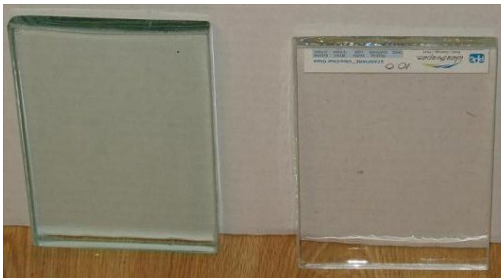
Figure 2: Image of regular glass on the left and Starphire glass on the right (courtesy of Glasscages.com).
