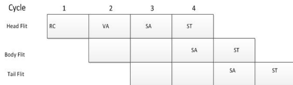
Figure 6. Router Pipeline Stages
