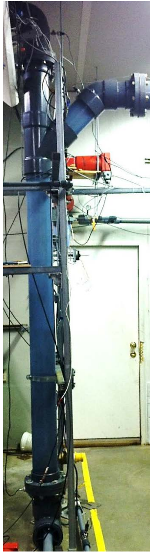
Figure 4.9. 6" Separator with Wye Pipe Fitting
