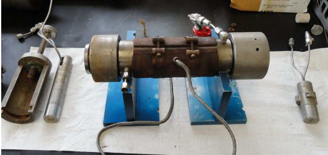
Fig. 2.7—Core holder assembly with 1-in. diameter by 6-in. length
