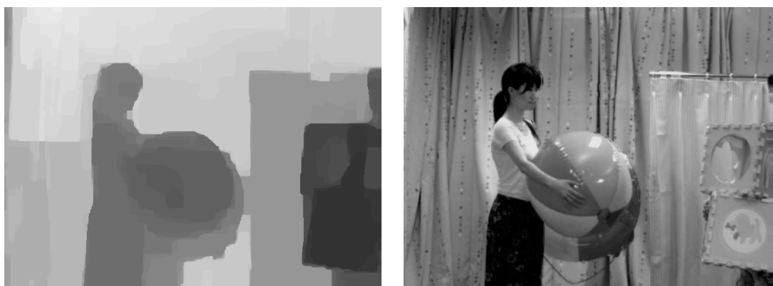
(a) The depth image of camera view 1 frame generated by DERS. (b) The side information frame for 35(c) warped from camera view 0 frame by DERS (PSNR 27.38dB).
