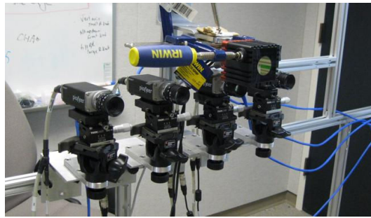
Fig. 31. The camera system setup for the collection of four correlated video sequences.
