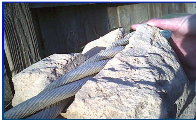
Fig. 2.2— Steel abrasive cable can cut through target formation (Carter, 2009).
