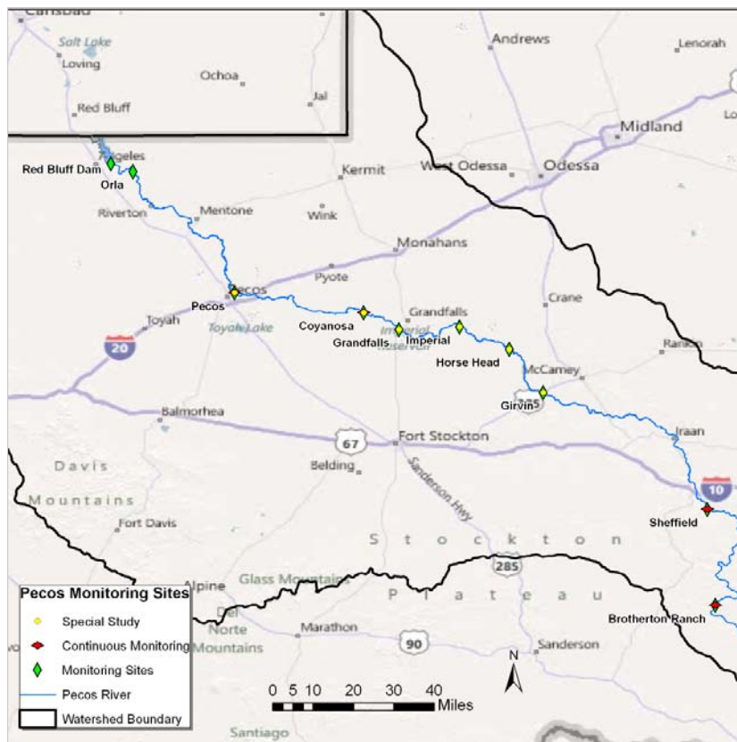
Figure 5. Monitoring stations on the Pecos River. These 10 stations provided various forms of surface water quality data for the salt load and geochemical analyses.
