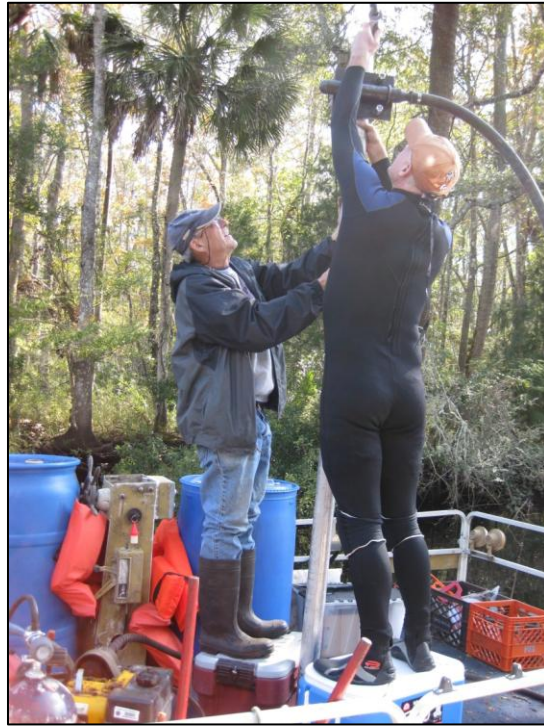
Figure 4.5. Vibrocorer head being placed on aluminum core tube in center of pontoon boat.
