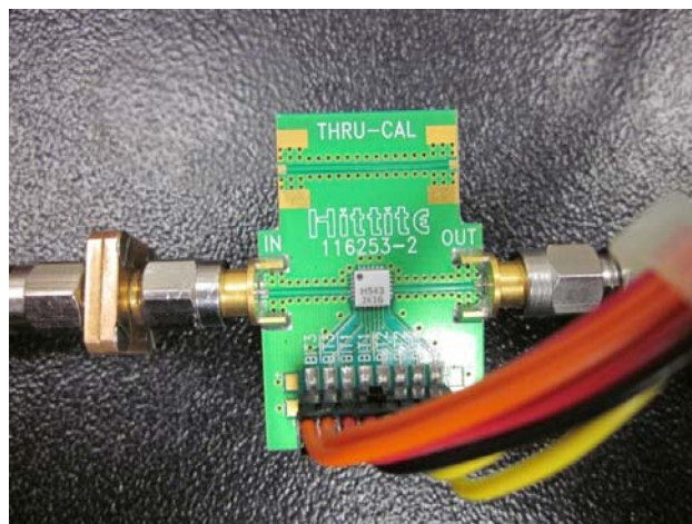
Fig. 8-19. Phase shifter measurement using network analyzer.
