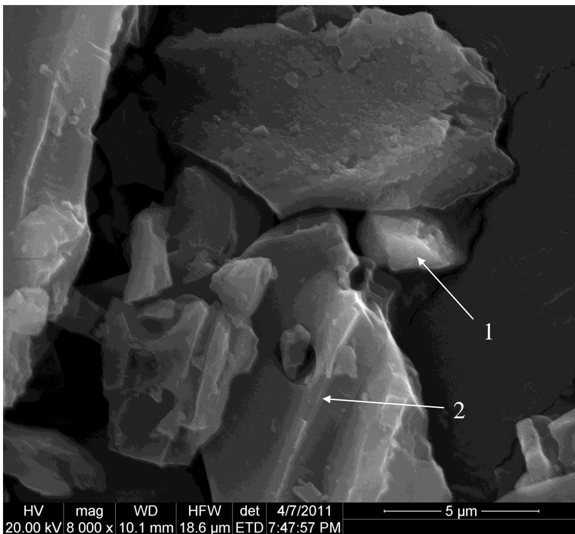
Figure 4: SEM Image of Non-Activated Biochar at 8000X Magnification from Which EDS Spectra Were Taken at Points 1&2
