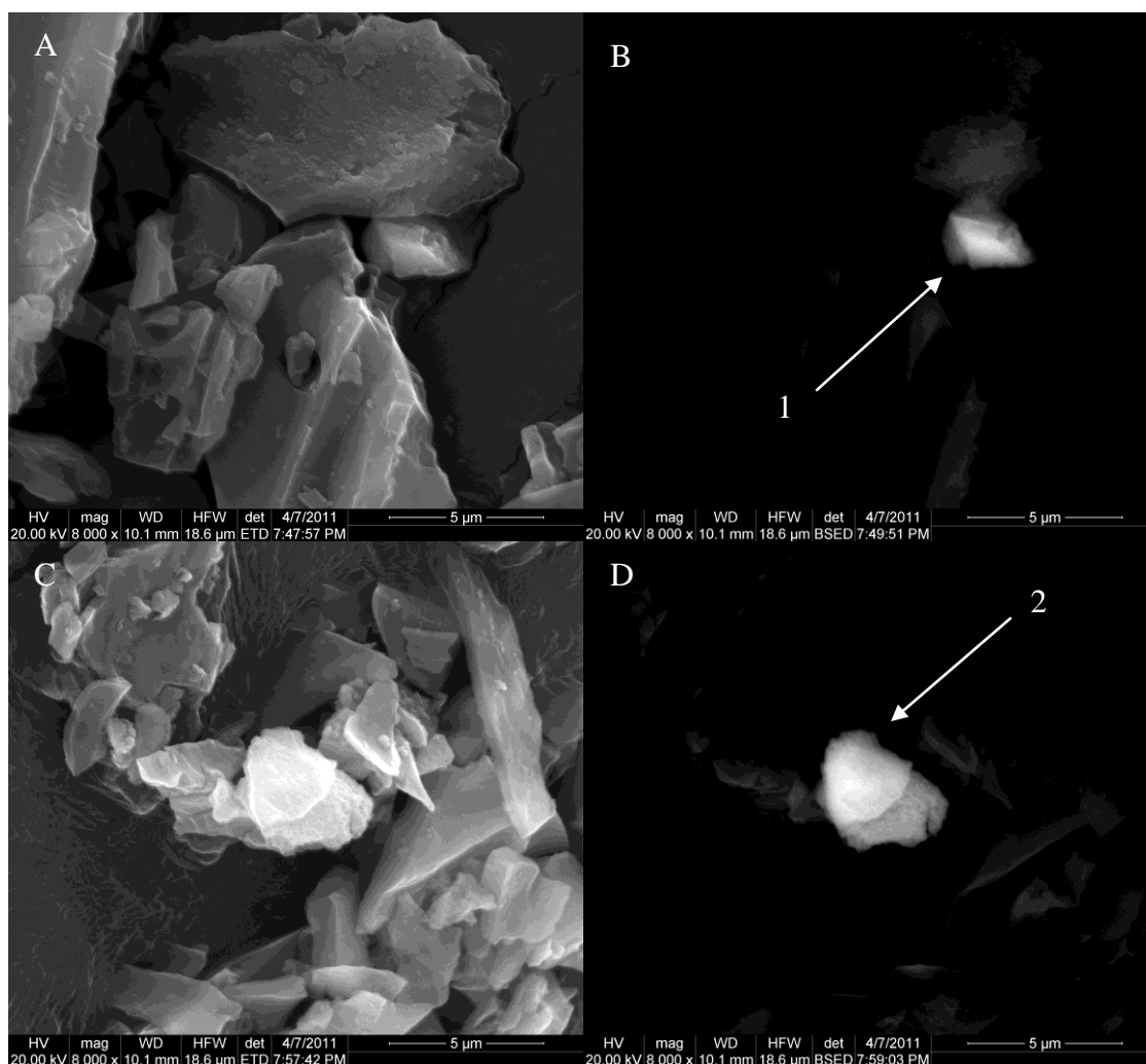
Figure 3: SEM Images of Non-Activated Biochar at A) 8000X, B) Backscatter View of Image A, C) 8000X, and D) Backscatter View of Image C
