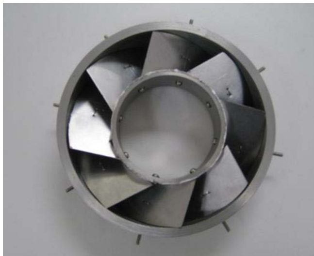
Figure 11: Swirler at 60^\circ swirl angle
