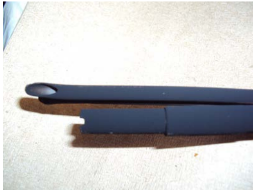
Figure 35: Soot formed on the sintered filter of analyzer probe
