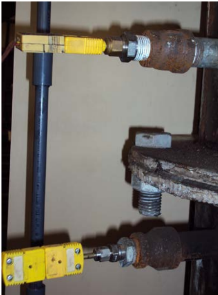
Figure 24: Thermocouples in chamber ports
