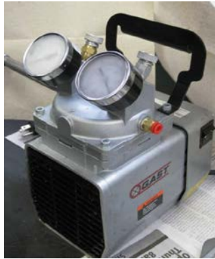
Figure 15: Primary air compressor
