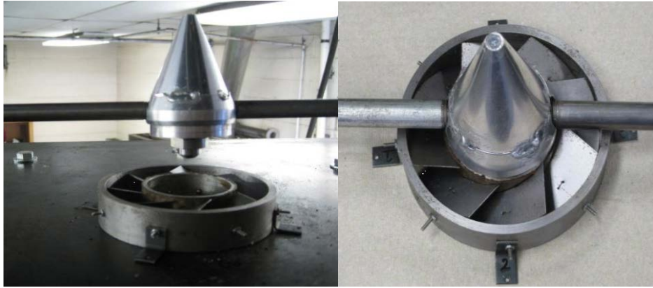
Figure 26: Nozzle with aluminum cone placed over the swirler
