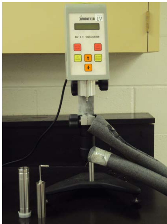
Figure 30: Brookfield Viscometer with UL adapter, spindle and cylinder
