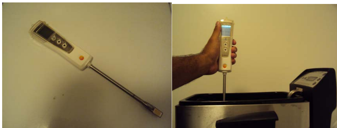
Figure 28: Testo 270 cooking oil tester, measuring TPM of corn oil in deep fryer
