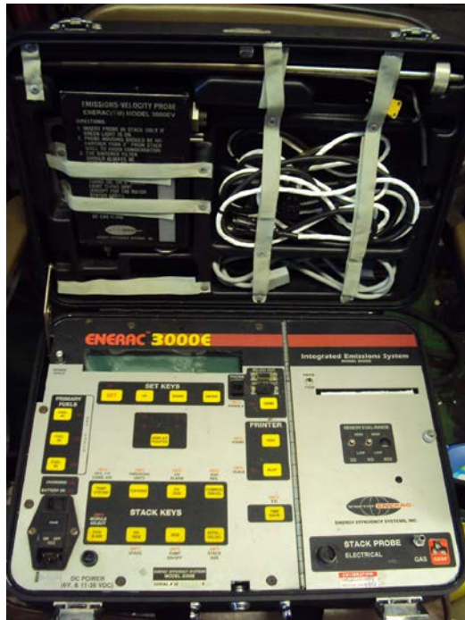
Figure 18: Emissions gas analyzer: Main unit (L) and probe housing (R)
