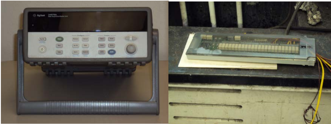
Figure 20: DAQ from Agilent and multiplexer card
