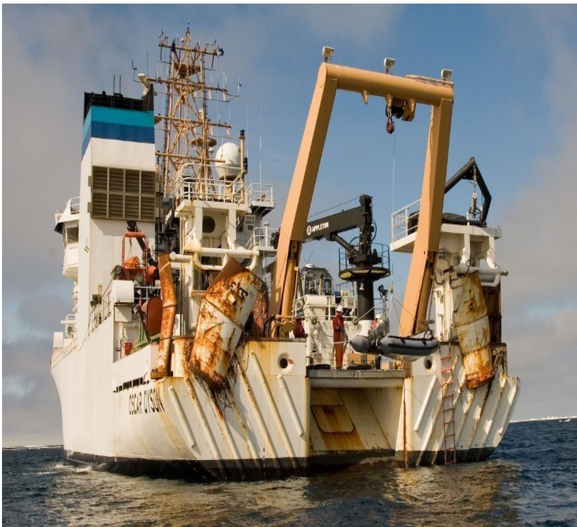
Figure 5. Stern ramp of the NOAA fisheries research vessel Oscar Dyson . (Courtesy of NOAA).
