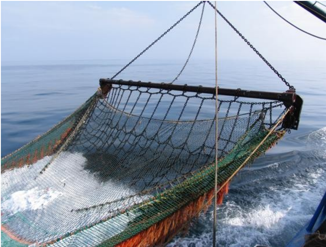
Figure 9. A beam trawl with chain mat. (Photo courtesy of The Institute for Agriculture and Fisheries Research).
