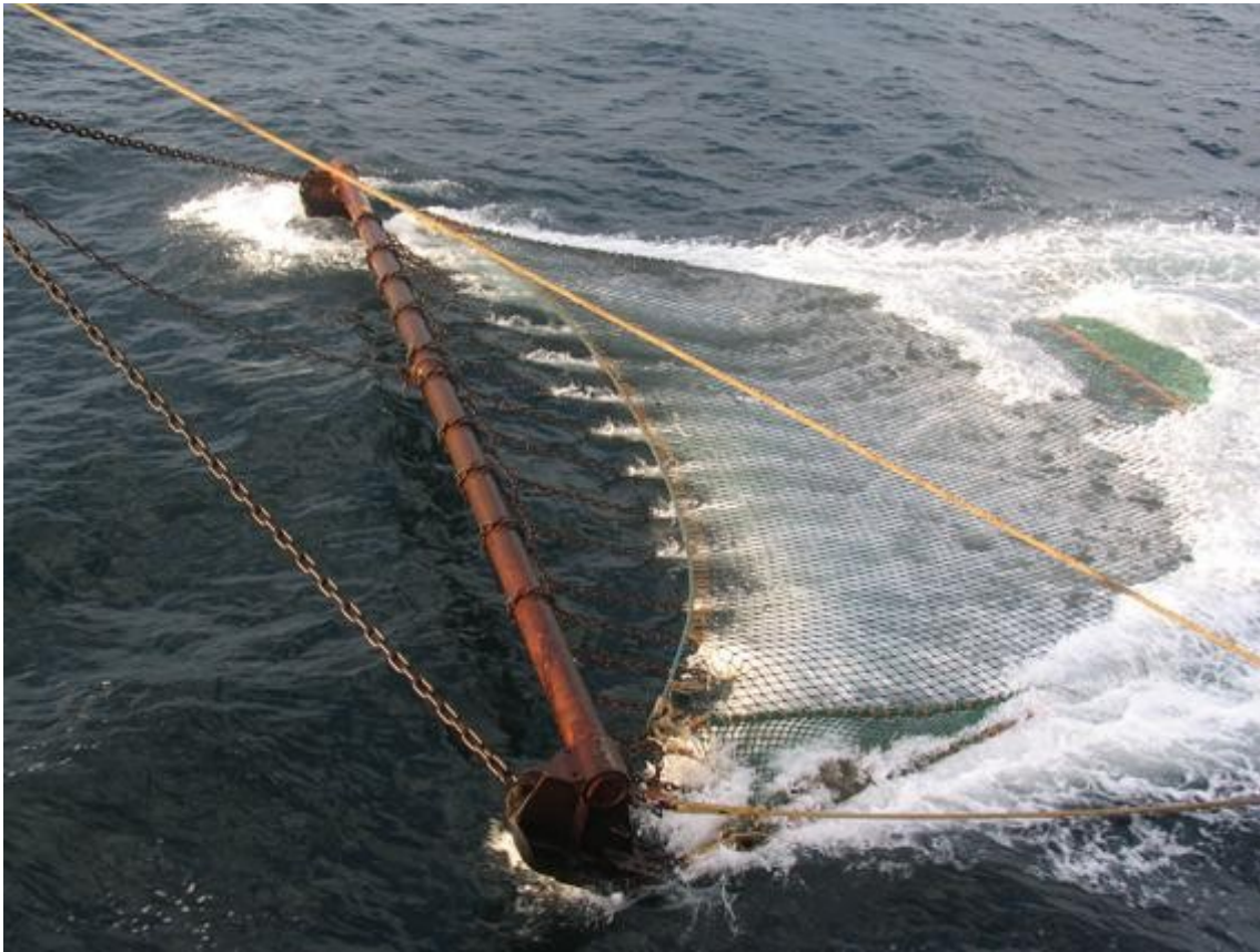
Figure 2. A beam trawl being set. (Photo courtesy of The Institute for Agriculture and Fisheries Research).
