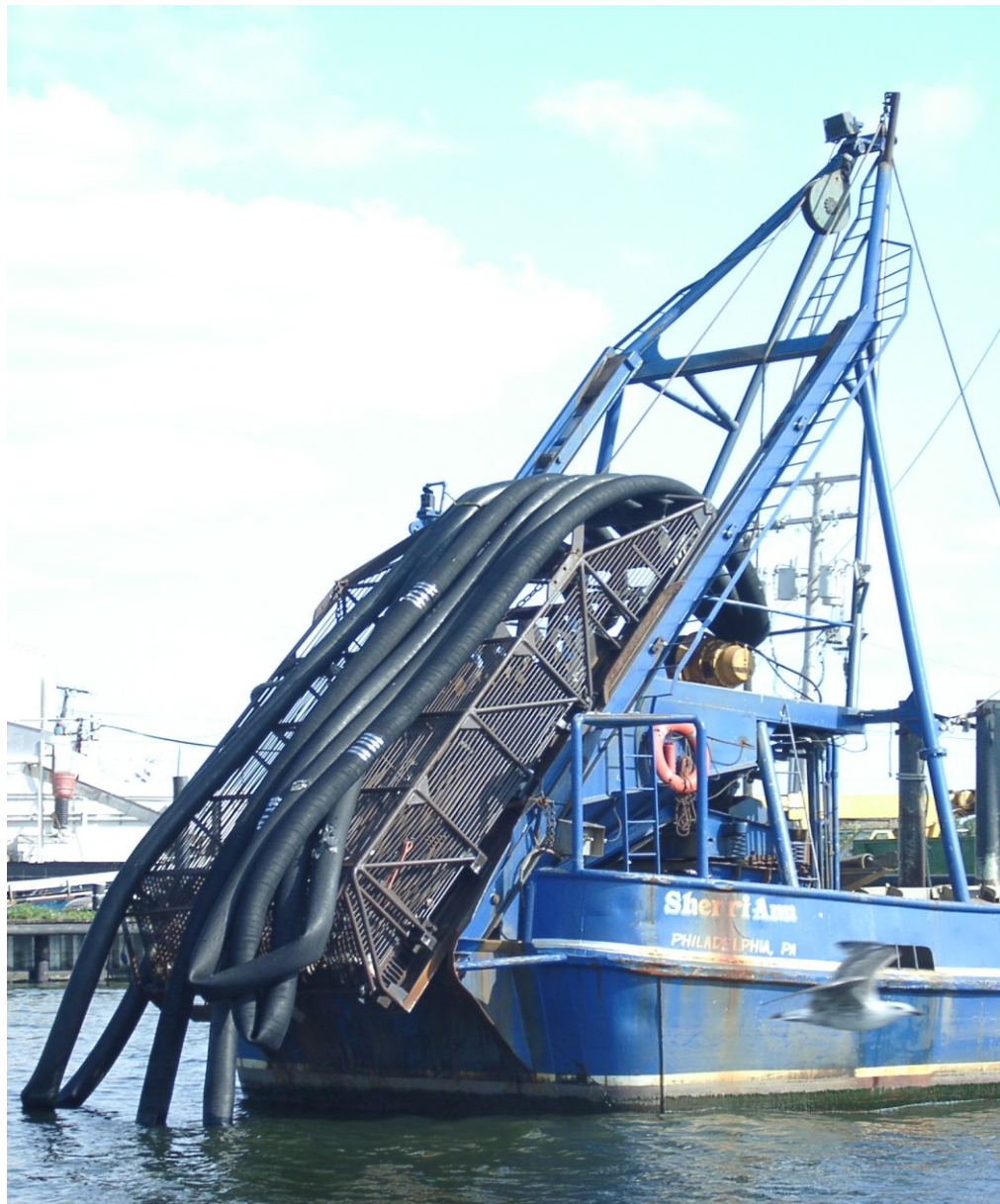
Figure 12. A large hydraulic oyster dredge on the Sherri Ann leaving Point Pleasant, NJ. (Photo by Rich Galiano).
