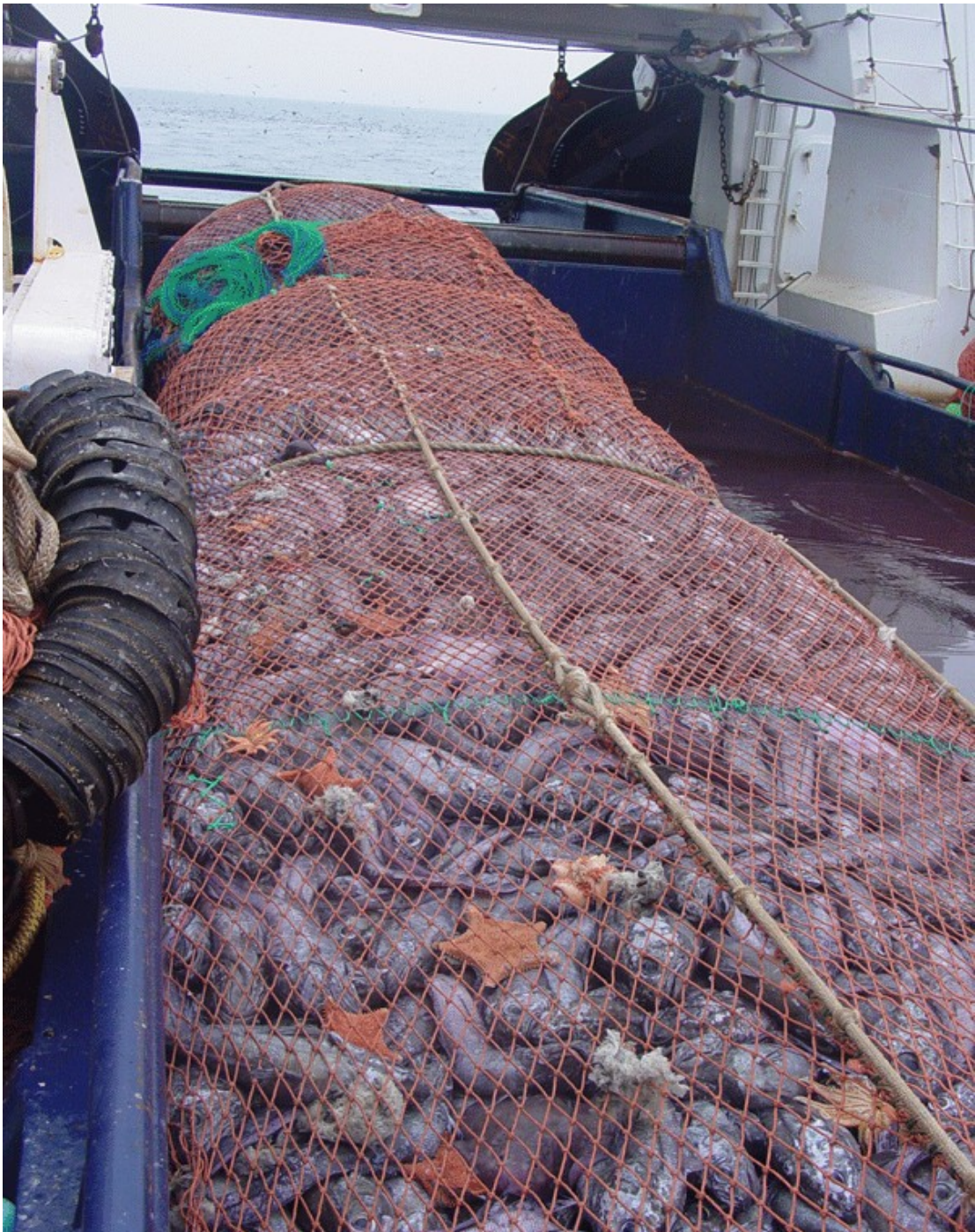
Figure 6. Full cod-end of an otter trawl after a research trawl. (Courtesy of NMFS/NOAA fisheries)
