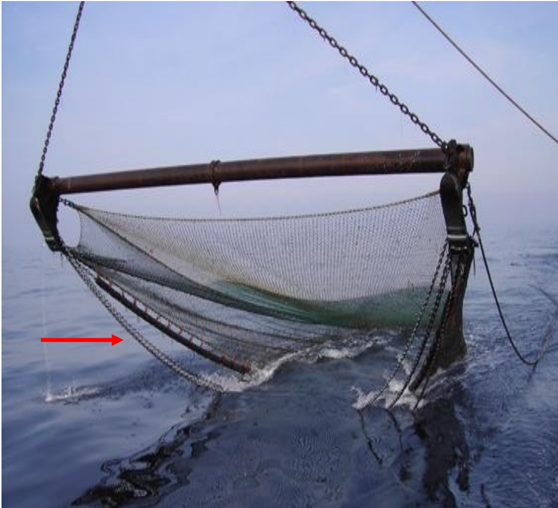
Figure 8. A beam trawl with tickler chains. (Photo courtesy of The Institute for Agriculture and Fisheries Research).
