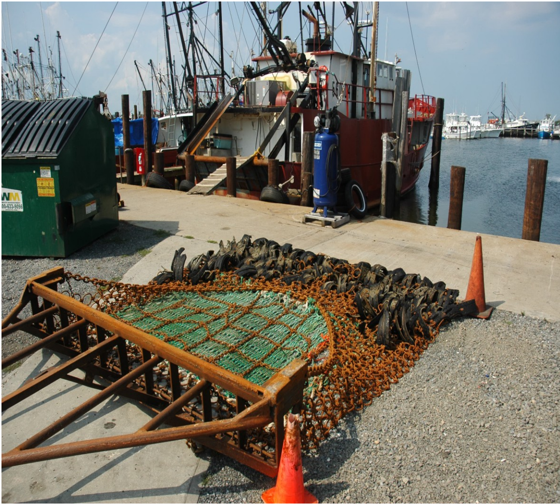
Figure 10. A scallop dredge with pieces of old tires to protect the ring mesh on the dock in Viking Village, Barnegat Light, NJ. (Photo by Rodd Halstead).
