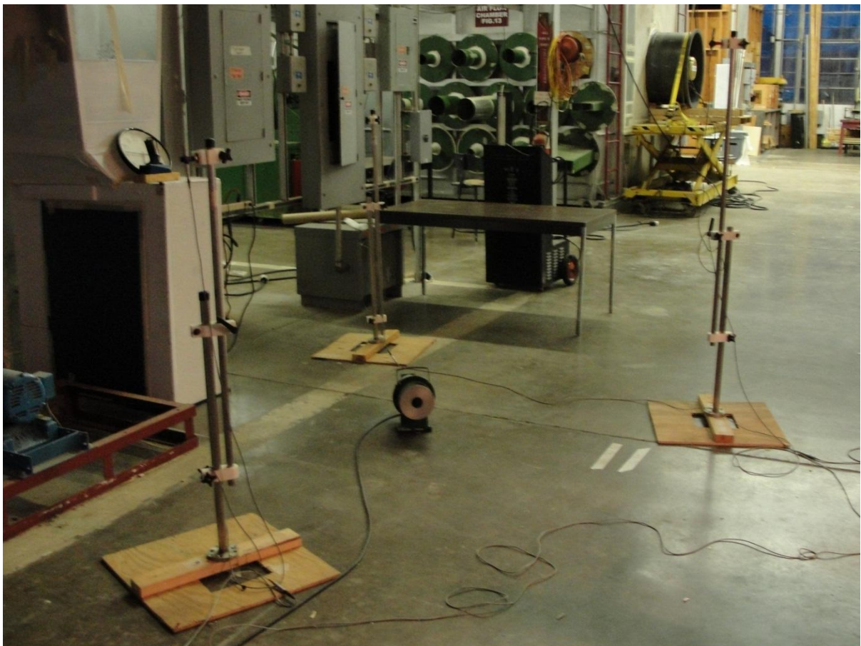
Figure 9. Transmission Loss Setup Outside the Semi-Reverberant Sound Chamber
