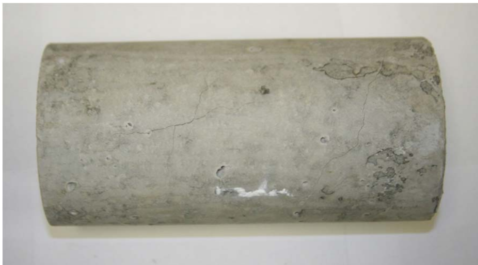
Figure 5-14. Cracking of a Cylinder Stored in the Curing Room [taken from Bracci et al. (2011)].
