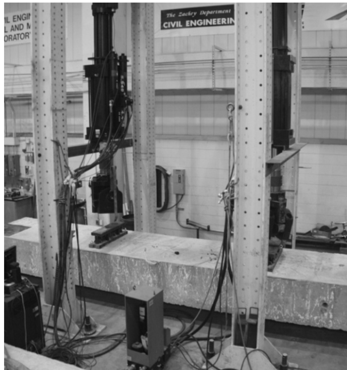
Figure 5-4. Specimen in the Four-Point Test Setup [taken from Alberson (2009)].
