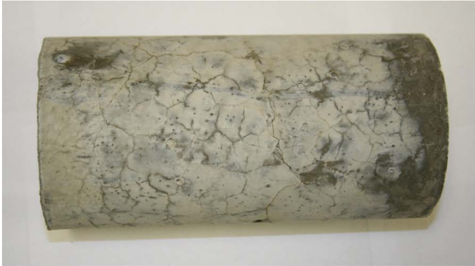
Figure 5-15. Cracking of a Cylinder Stored at the Riverside Campus [taken from Bracci et al. (2011)].
