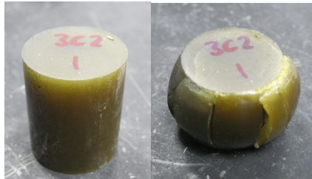
Fig. 32—A specimen of fully cured resin mixed with 2000 pipe dope before and after the compression test
