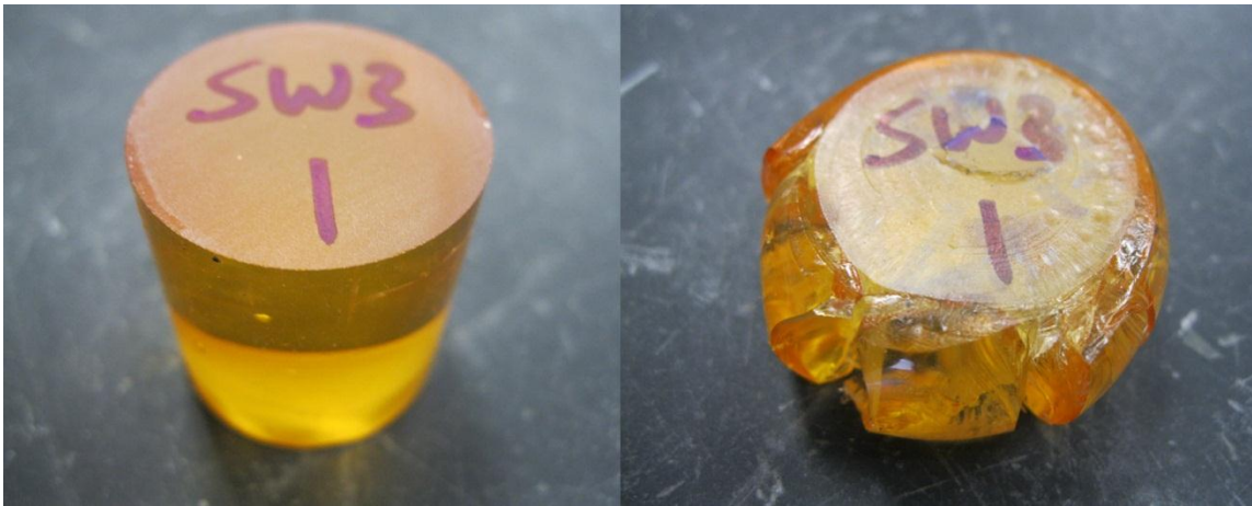
Fig. 20 —A specimen of fully cured resin mixed with seawater brine before and after the compression test
