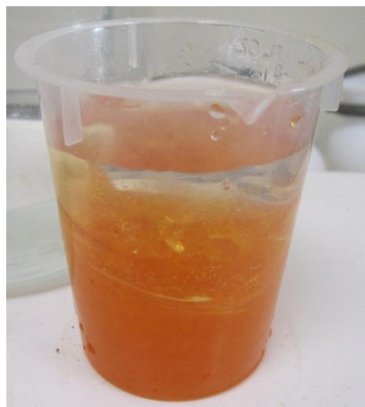
Fig. 16—The separation of resin and seawater brine is apparent due to the fluids being immiscible
