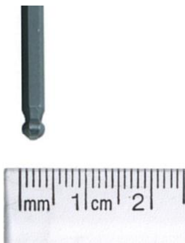
Fig. 49 —The 3mm metal rod used in the qualitative level of gelation test
