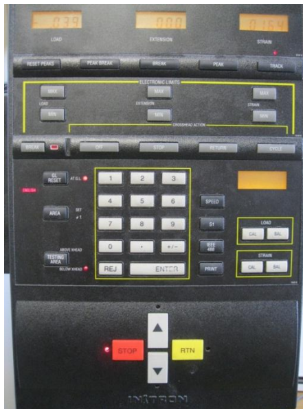
Fig. 13—The control panel for the Instron 4206
