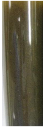
Fig. 30—The fully cured sample of resin mixed with 2000 pipe dope
