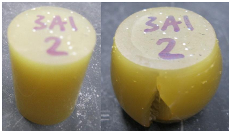
Fig. 24 —A specimen of fully cured resin mixed with ZN18 pipe dope before and after the compression test
