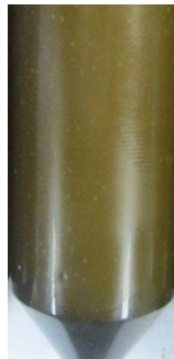
Fig. 34—The fully cured sample of resin mixed with OCTG pipe dope
