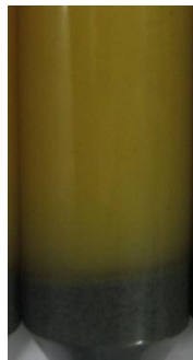
Fig. 42—The fully cured sample of resin mixed with 4010NM pipe dope
