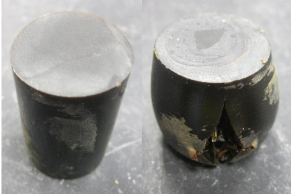
Fig. 47—A specimen of fully cured resin mixed with oil before and after the compression test
