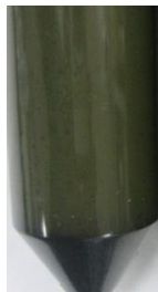
Fig. 38—The fully cured sample of resin mixed with Metal-free pipe dope
