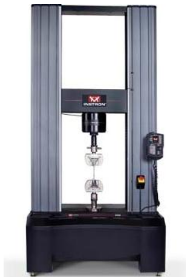
Fig. 12—The Instron 4206 used for compression tests with a load limit up to 30,000 psi
