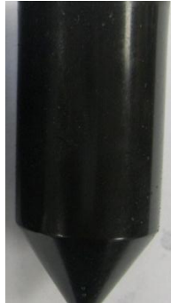
Fig. 45—The fully cured sample of resin mixed with sour oil
