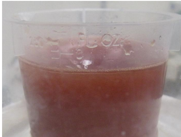
Fig. 17 —An emulsion of resin droplets in seawater brine during and after mixing for one hour prior to curing
