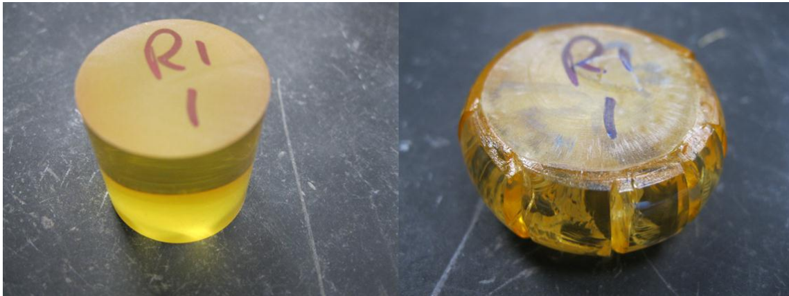
Fig. 15—A specimen of pure epoxy-based resin before and after the compression test
