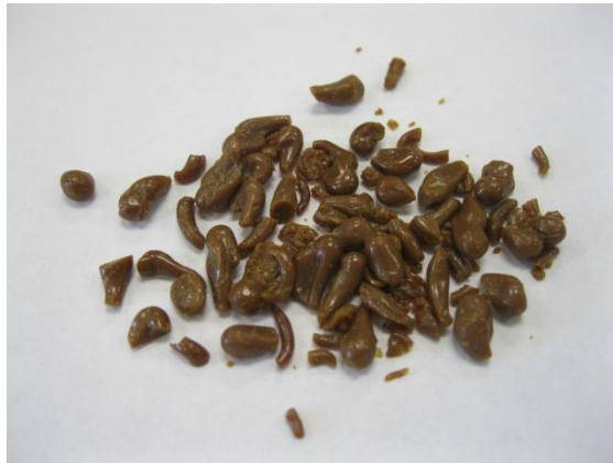
Fig. 62—Vitrified resin droplets that were formed by quenching droplets of resin in 39°F water 3.5 hours into the cure process
