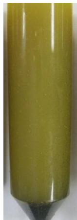
Fig. 22—The fully cured sample of resin mixed with ZN18 pipe dope
