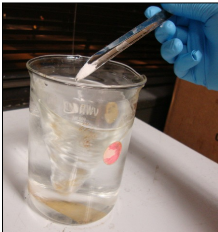
Fig. 14 - Careful Addition of HPAM to Water
