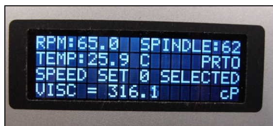
Fig. 42 - Viscosity Reading Displayed on Brookfield DV–III Ultra Rheometer
