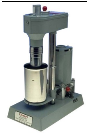
Fig. 64 - Fann – 35 Viscometer (Fann Instrument Company)
