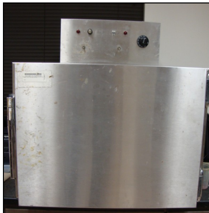
Fig. 22 - Oven Used to Test Gel Samples at 200 °F
