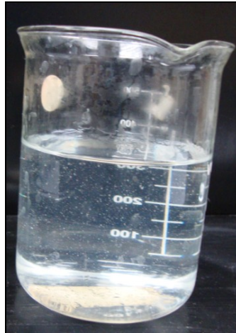
Fig. 18 - HPAM/ PEI (Research Grade) Gelant Solution. Clear in Appearance
